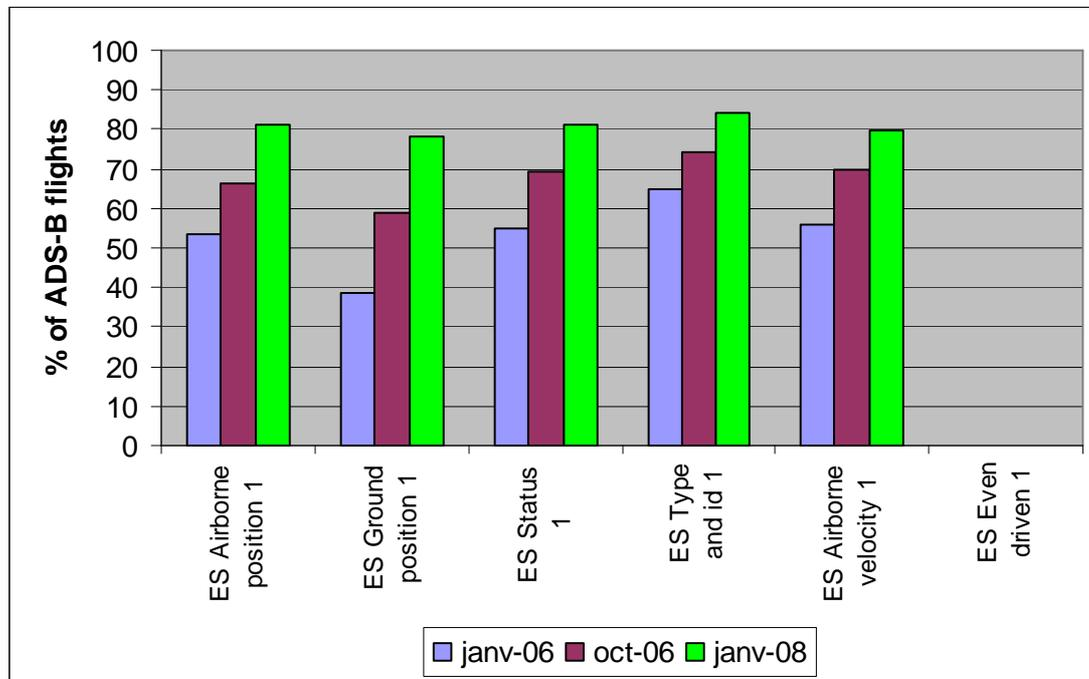
**Figure 1 Statistics for Extended Squitter capable flights**
