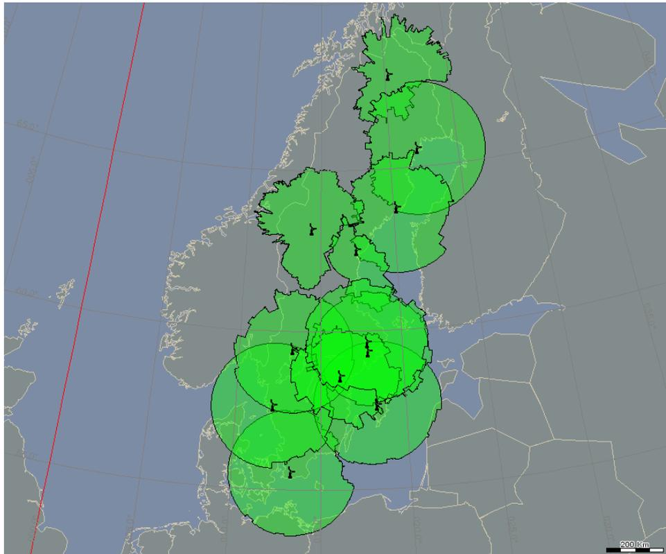
**Figure 3 Estimated coverage at 10,000 ft above Mean Sea Level for the Swedish ADS-B network when all 12 ground stations are deployed (Analysis done using EUROCONTROL CAPT tool)**
